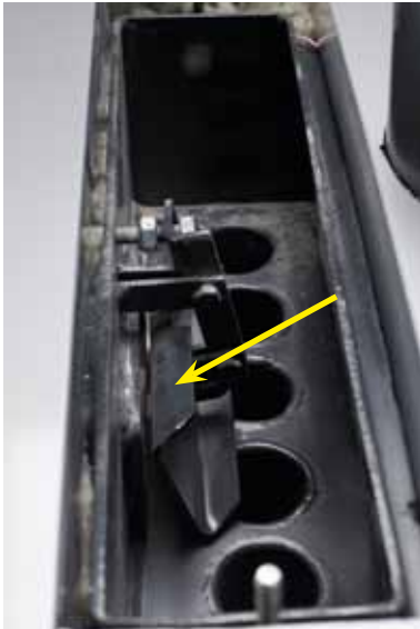
Make sure that the fire door damper opens and closes as you use the feeding hatch.
