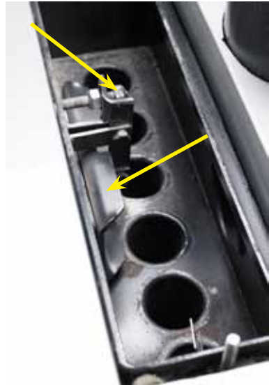
Make sure that the fire door damper closes when you close the feeding hatch.
