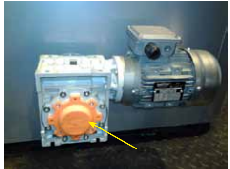
Install the bearing cover plate.
