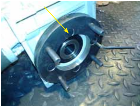
Install the motor adapter flange with four M8x25 countersunk screws.
