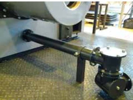
Ash screw with extension piece.
